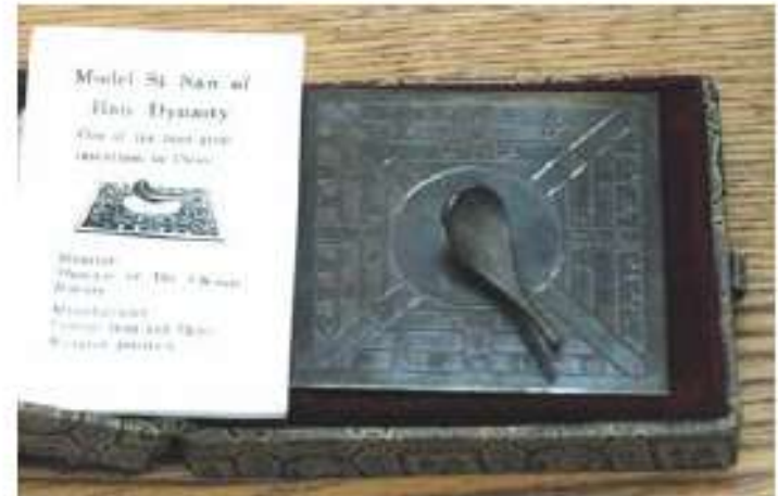
Model of compass used in China about 450 BC. The reference direction was south
