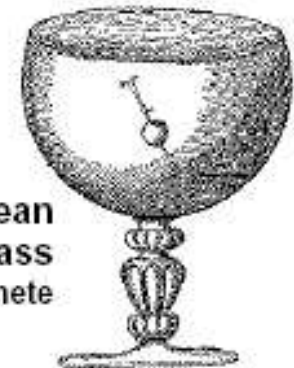
Model of compass used in China about 450 BC. The reference direction was south
